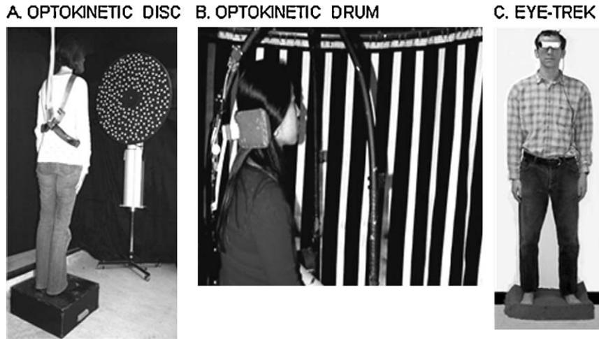
**Fig. 2.** Apparatus and sample exercises for the simulator-based intervention. (A) Optokinetic disc: a subject focuses on the black circle in the disc's centre while the disc rotates. (B) Optokinetic drum: the subject is seated in the stationary chair and asked to stare ahead while the drum rotates. (C) Eye-Trek: a subject stands on foam while viewing a visual motion scene with the Eye-Trek device. The velocities of motion employed are explained in Section 2.
